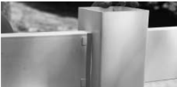
Country Estate rails utilize wedge locks that allow expansion without uncoupling, once pushed through the routed post opening.
